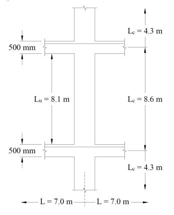
Figure 2 – Slender Reinforced Concrete Column Elevation
