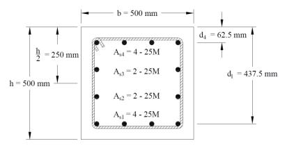
Figure 1 – Slender Reinforced Concrete Column Cross-Section
