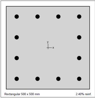
Figure 1: Column section
