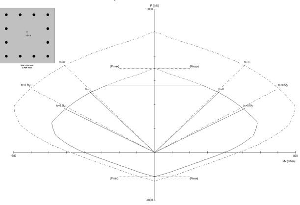
Figure 6 – Designed Column Interaction Diagram
